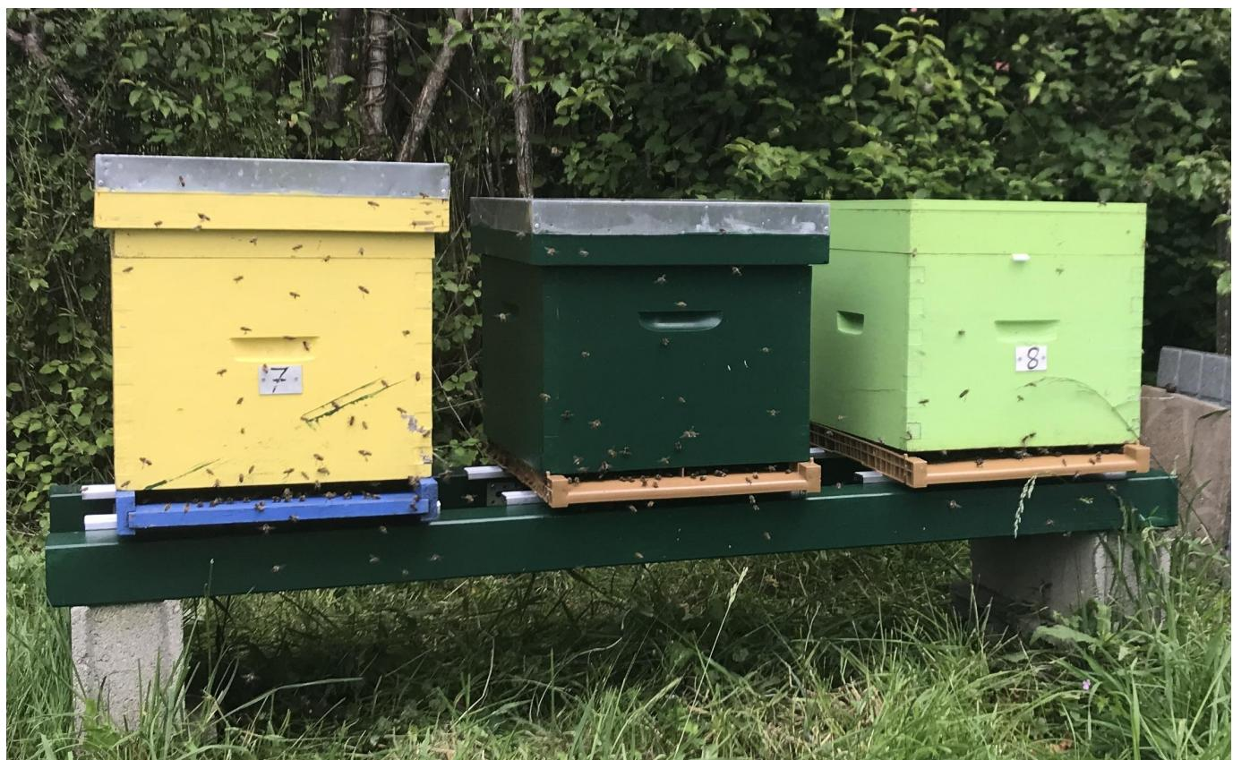
The Multiscale2 system utilizes a single XLR board and two 100 kg load cells per hive, enabling independent weight measurement for up to four hives.
