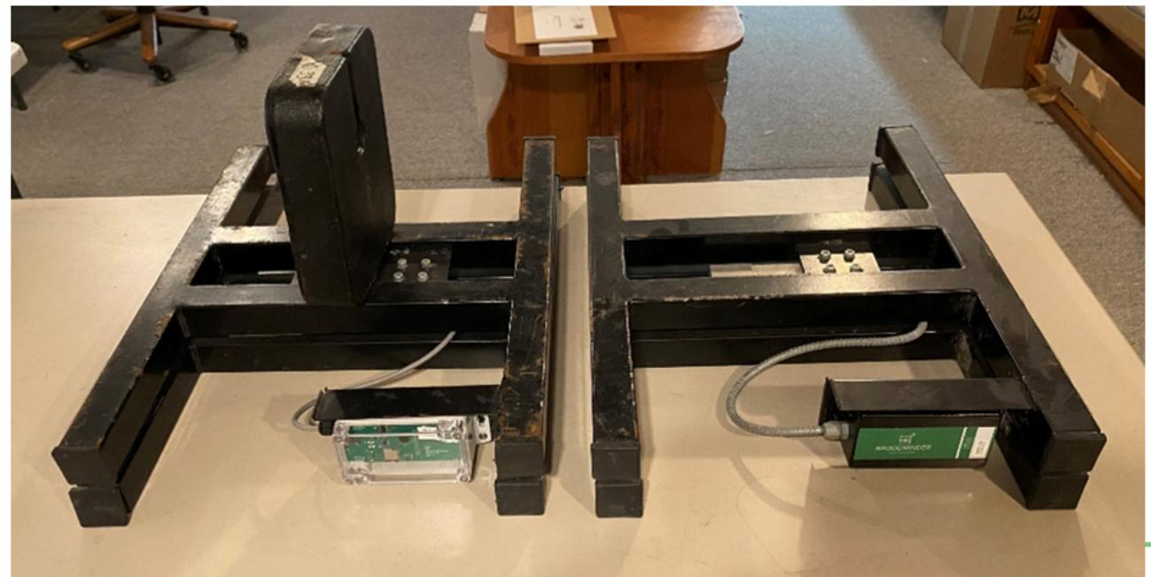
10. The BLE chip will work better if it is oriented so the circuit board is away from the metal frame.
