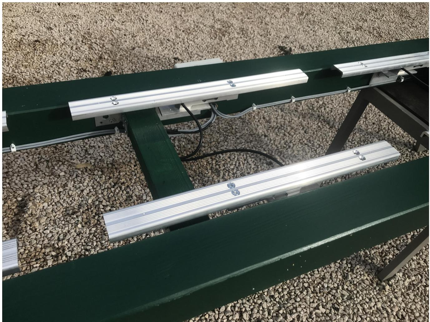
We're using W4 bars as top support and 100kg loadcells (one at the front and another at the rear). They are hooked to the wooden structure with an L shaped 5mm aluminium profile.
