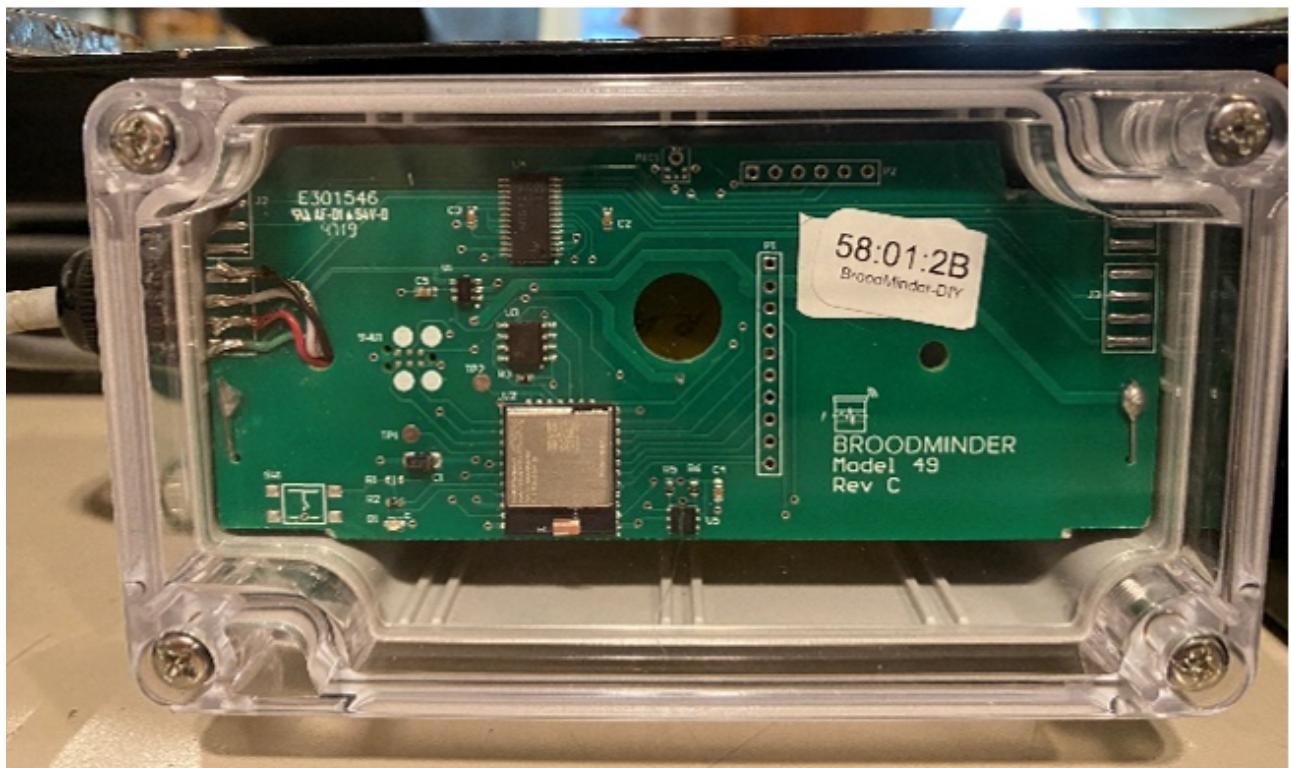
9. If the box is tucked up in good spot, you might be able to get away with mounting without sealing the cable entry. Be certain to have a drip loop so that rain doesn't drip inside.
