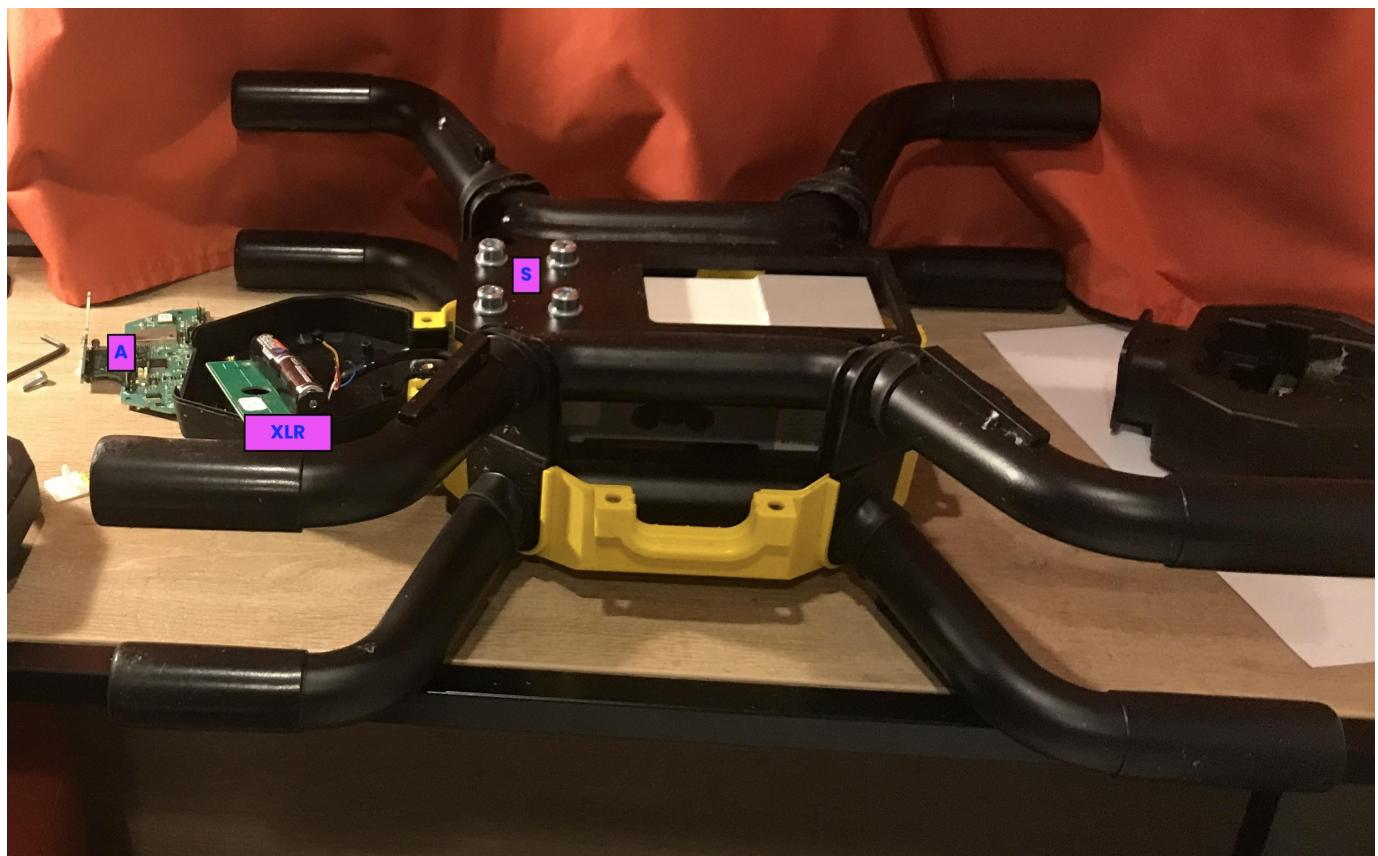
In the box remove the "A" board and the "B" harness. Unscrew the "C" harness from the board. This is the one coming from the load-cell to be soldered on the new XLR board.
