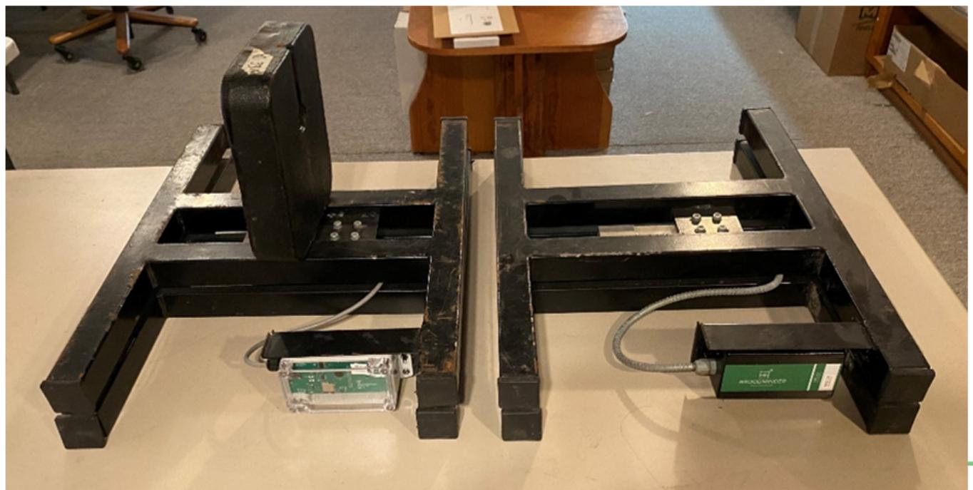
It is easy to take an old broken hive scale and convert it to a BroodMinder enable scale. Here is an example.
