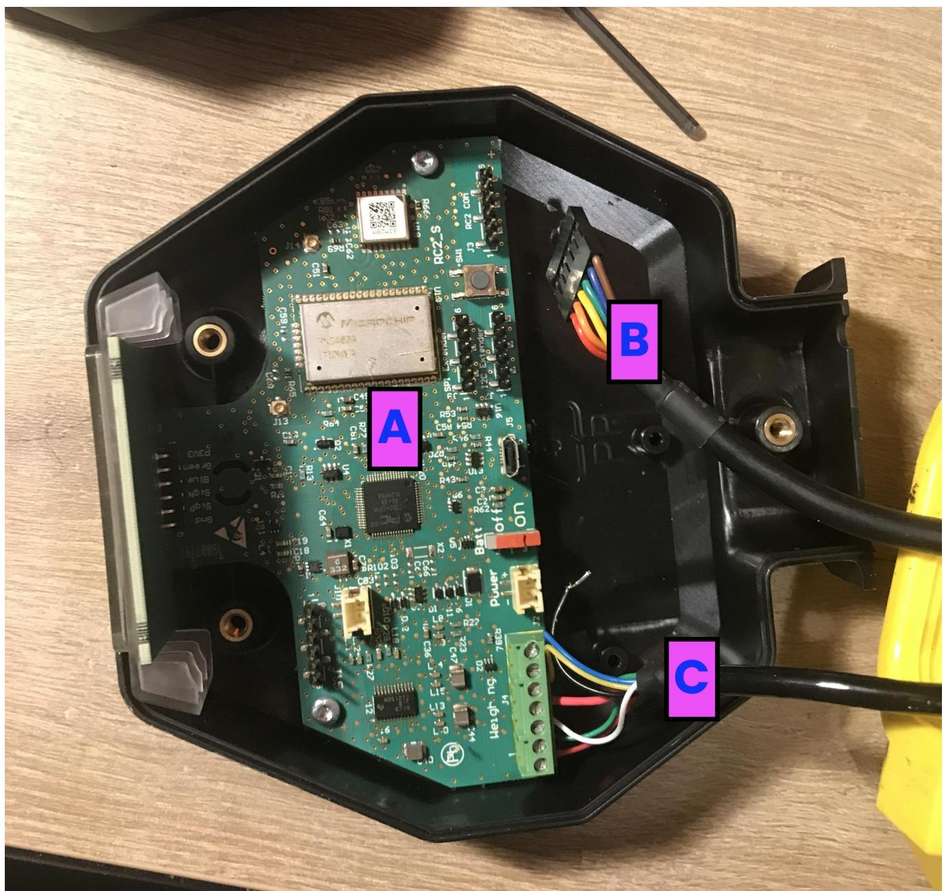
Now cut the central plot with a cutter to leave space to the XLR board
