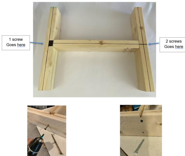
To assemble your frame, make sure you have a flat surface and ensure your pieces are square. Follow the picture above for the correct orientation of the boards.
