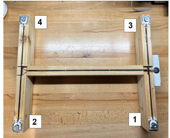
Use 4 "C" screws per sensor. Make sure that before you drill in the sensors to the wood that you put the load cell custom support () between the sensor and the wood to allow for the sensor to read correctly. If the mount is not installed, it can cause the sensors to record incorrect information.
